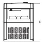
Figure 8-2 Physical appearance and overall dimensions of the H300 (sheet metal housing)
