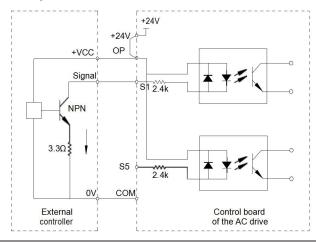
This is the most commonly used wiring mode. To apply external power supply, remove jumpers between +24 V and OP and between COM and CME, and connect the positive pole of external power supply to OP and negative pole to CME.
